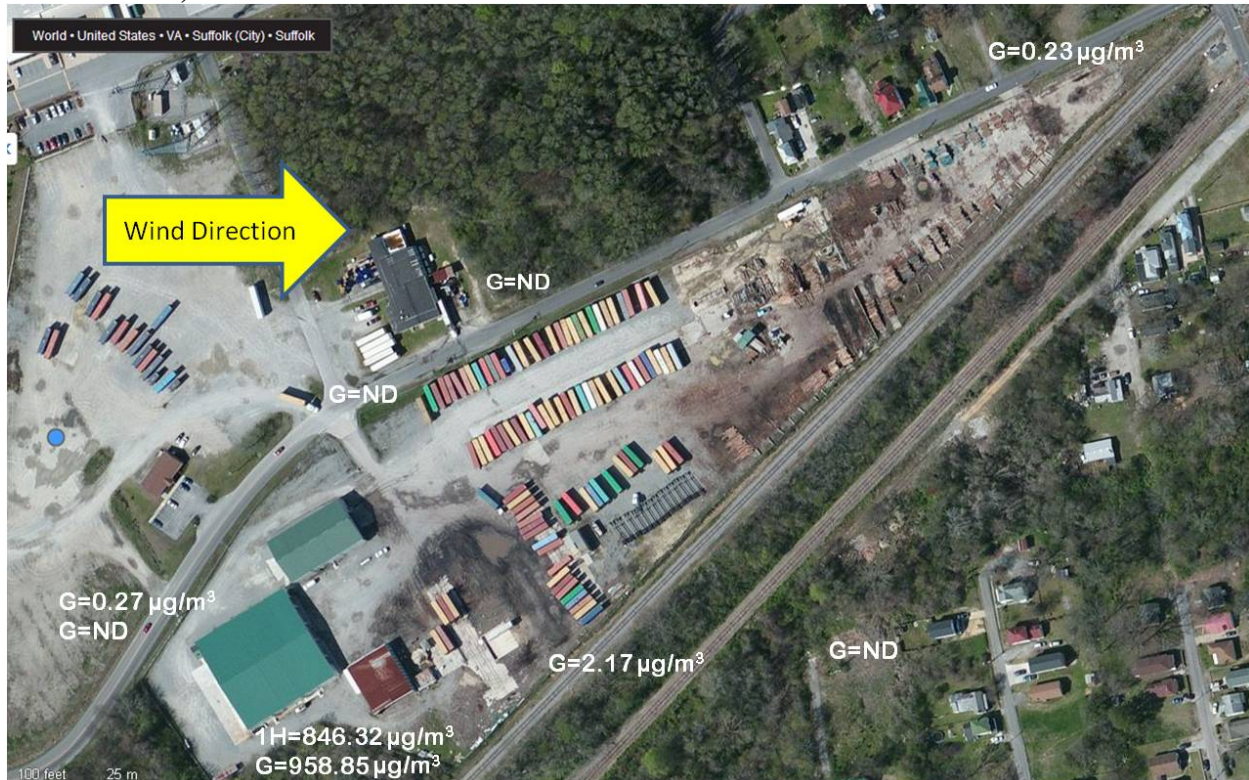
Figure 2. Methyl bromide air concentrations collected during aeration at Royal Fumigation on March 19, 2010.*
