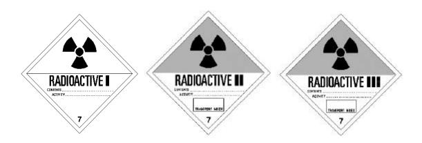
For all labels, vertical bars on each label are in red. Each label is diamond-shaped, four inches (10 cm) on each side, and has a black solid-line border one-fourth inch from the edge. The background color of the upper half (within the black line) is white for the "I" label. It is yellow for the "II" and "III" labels. The regulatory provisions of §§172.403(f) and (g) that apply to the use of these labels are indicated below.
