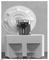
Figure A-Molybdenum 99 Generator
