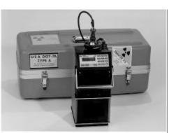
Figure B-Moisture Density Gauge & Carrying Case
