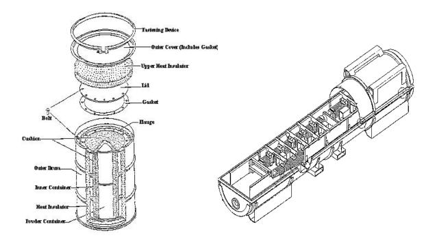
Figure A-Type A Drum for  $UO_2$
