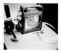
Figure B-Industrial Radiography Exposure Device
