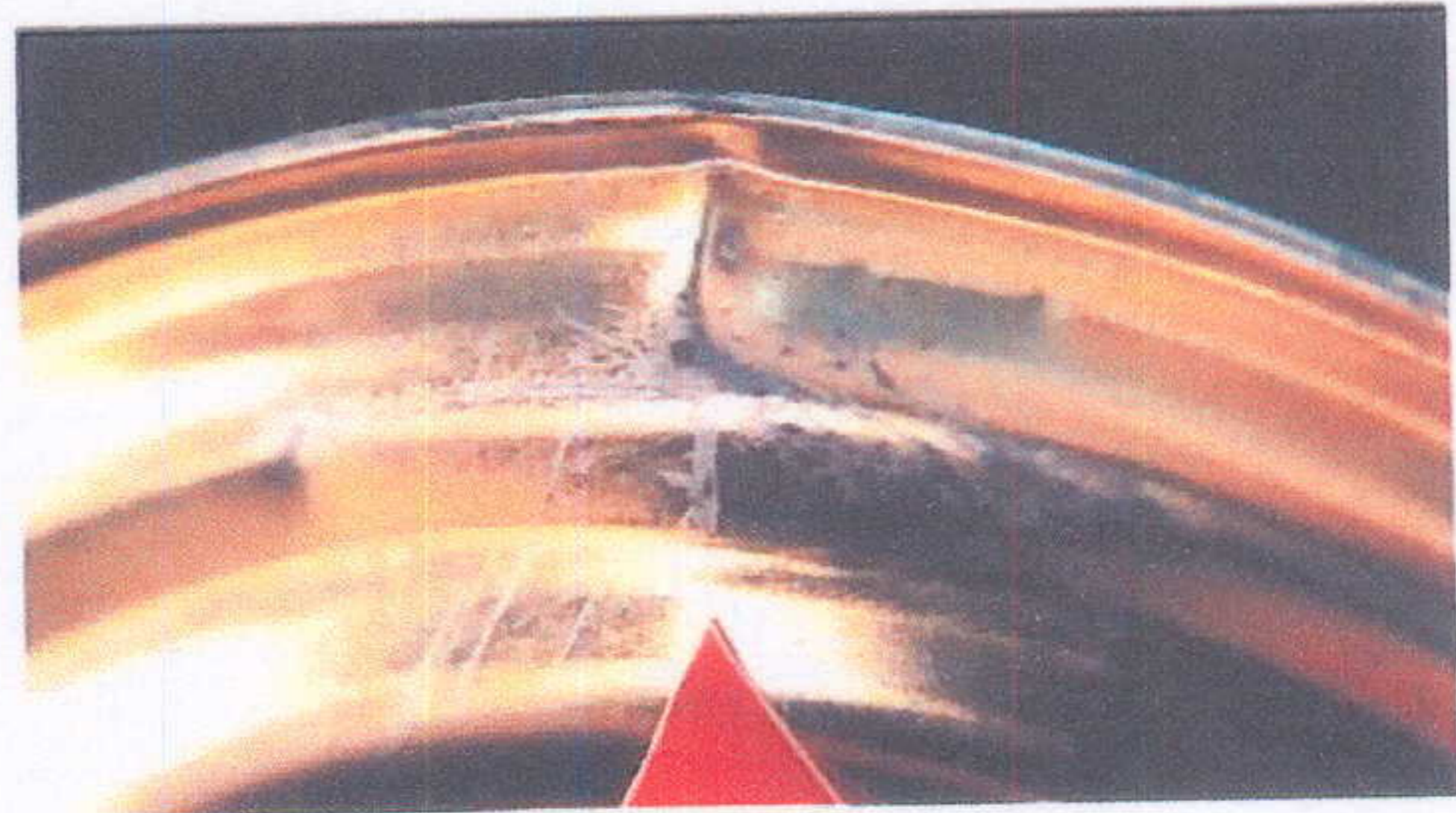
21. Minor "buckle" just extending into double seam on end of can body (Double seam does not appear significantly affected.)
