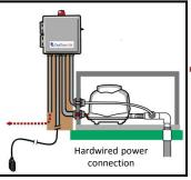
Fuji Clean allows FujiMAC "R" series blower power connection to be either via outdoor rated outlet or hardwired to control panel. Some states and jurisdictions require hardwire connection. Please check with local regulations.
