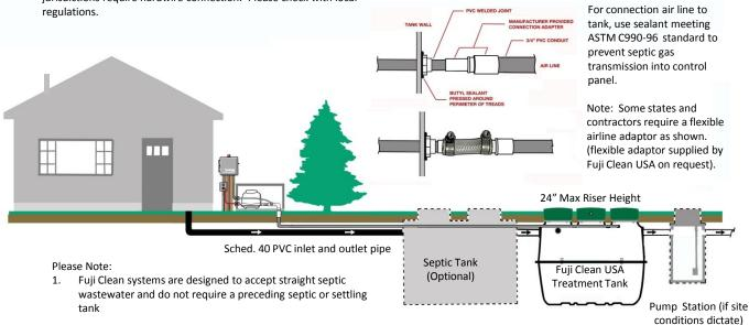
"Clearwater" water softener backwash should be discharged directly to footer (if regulations allow) or diverted around Fuji Clean system to drainfield.
