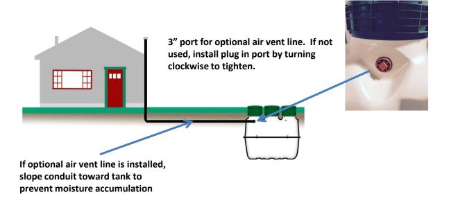
Step 13: During final landscaping, seeding etc., be sure to pitch final grade away from covers to sweep surface water away from treatment tank.
