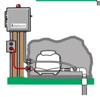
Two possible blower protection options. Be sure to <u>vent</u> covers to allow free air draw even in deep snow pack. □ Step 8: Locating and Installing Blower/Control Panel.
