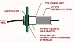
For connection of float switch cord to alarm panel, drill hole in riser and use male fitting and electrical conduit. Plug fitting with sealant standard that meets ASTM C990-96 to assure water-tight seal and to prevent septic gas transmission into control panel.
