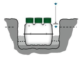
Step 6: Backfill about ¾ way up tank in layered, compacted 6" lifts using peastone or equivalent material that form-fits into tank corrugations. □ Step 7: Using supplied adaptors and fittings, attach air pipe fitting to tank and connect to ¾" conduit in prepared trench (min. 6" deep) to location of air blower. Please note: ¾" flexible irrigation line, 100 PSI Max, may also be used for the airline.
