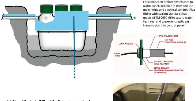
**Step 10:** Install Float Switch on pumpback line in  $2^{nd}$  chamber with 3-1/2'' tether. Float switch electrical cord should exit riser wall through male adaptor (caulked watertight to prevent gas leakage) or watertight fitting. An interior connection to direct burial cable is also acceptable.
