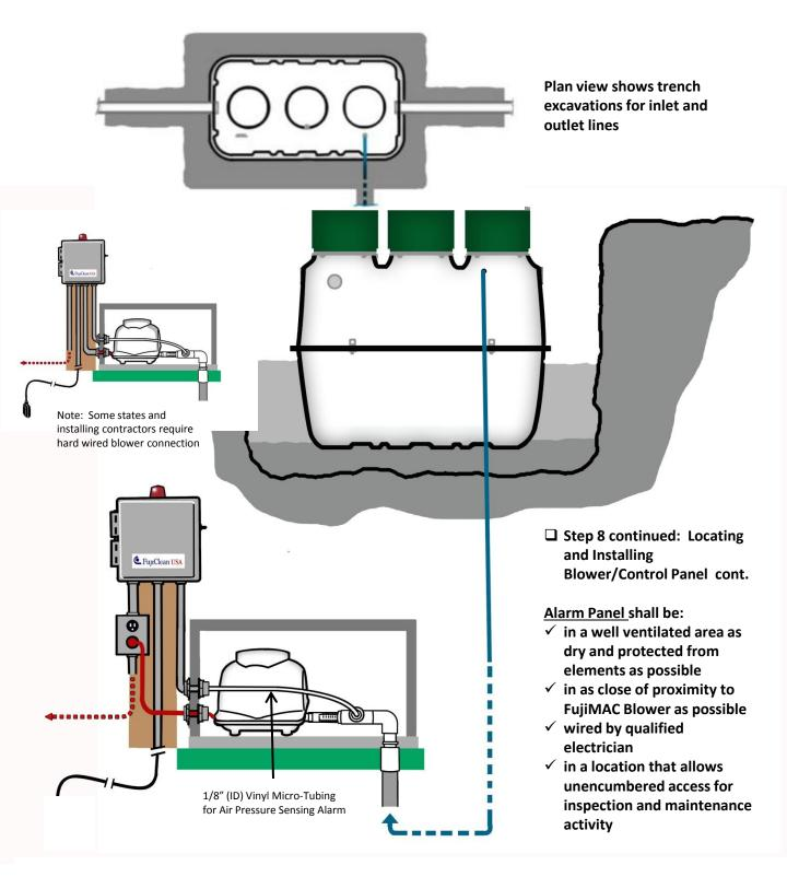
For additional important detail about installing and maintaining blower, please review and refer to provided <u>FujiMAC Blower Installation-Maintenance Manual</u>, which is provided inside the blower <u>box</u>. Step 9: For cold climate installations, please install insulated risers and covers and cover upper half of treatment unit with min. R-8 value insulating material (i.e. foam board)
