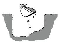
Step 1: Prepare excavation to be at least 1 to 2 feet larger than Fuji Clean system dimensions as listed below. Important Note: Riser height should not exceed 24".
