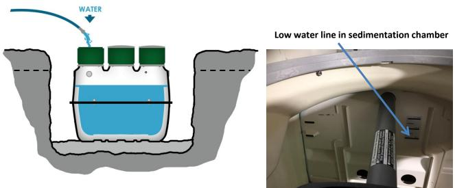
Please note: To assure tank water tightness, please check in 24 hours to be sure that the water level has not dropped. Please contact your distributor or Fuji Clean USA if water level has dropped.
