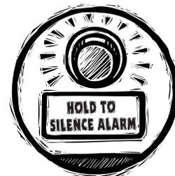
**Do** remember that the audible alarm can be silenced by pushing the lighted button located directly above the “Push to Silence” label on the front of the electrical control panel. With normal use, the tank has a reserve storage capacity good for 24-48 hours.
