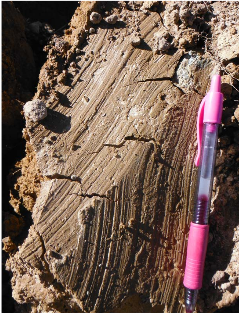
Figure: 6-17. Slickensides indicate the presence of smectitic clays that have a high or very high potential for shrinking and swelling. (Photo by Tom Saxton)
