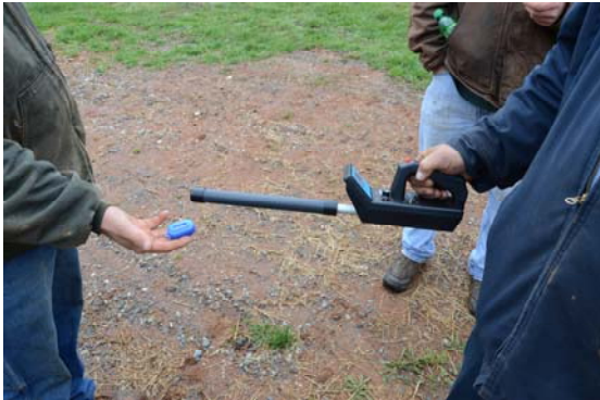
Figure: 7-7. A “mouse” may be used to locate the septic tank. It can be flushed down the toilet and traced. (Photo by Tom Saxton)
