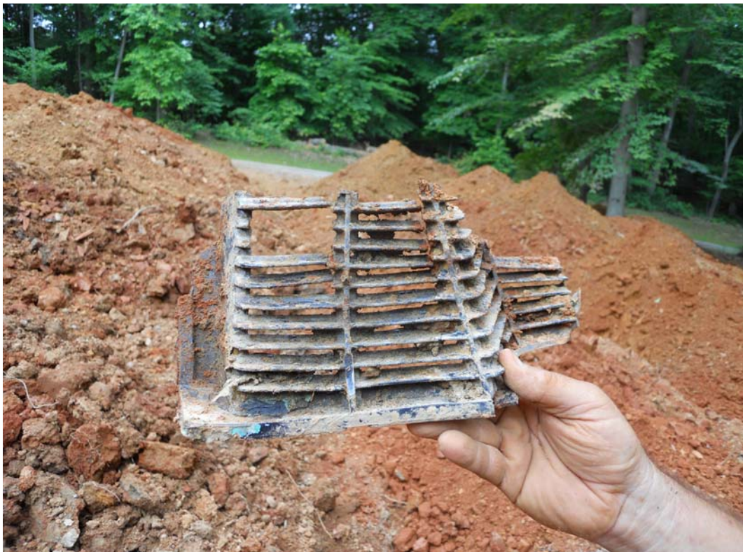
Figure: 7-22. The louvers in the chamber sidewalls allowed liquefied soil to slowly migrate into the void beneath the chamber. (Photo by Sarah Lewis, EHS)
