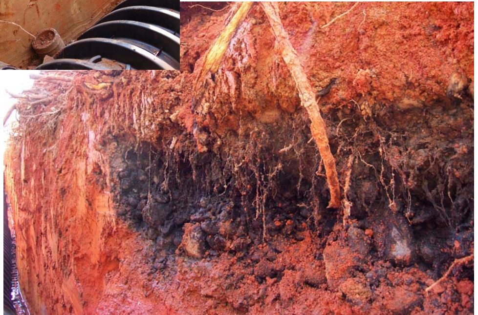
Figure: 7-27. Roots (above) and anaerobic conditions (below) due to poor septic tank maintenance and a perched water table have shortened the lifespan of these drainfields. (Photos by Tom Saxton)
