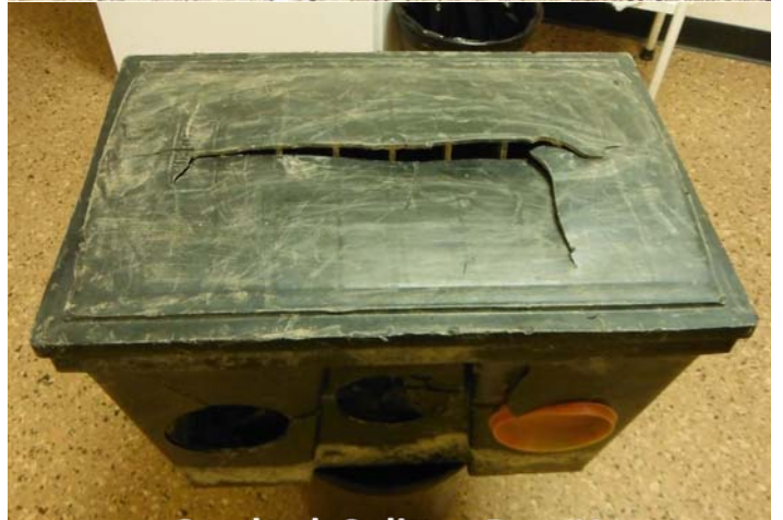
Figure: 7-34. Crushed plastic distribution boxes. (Photo by Tom Saxton)
