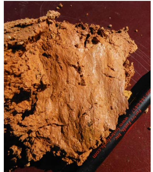
Figure: 6-18. Pressure faces may also indicate shrink swell soils. (Photo by Tom Saxton)
