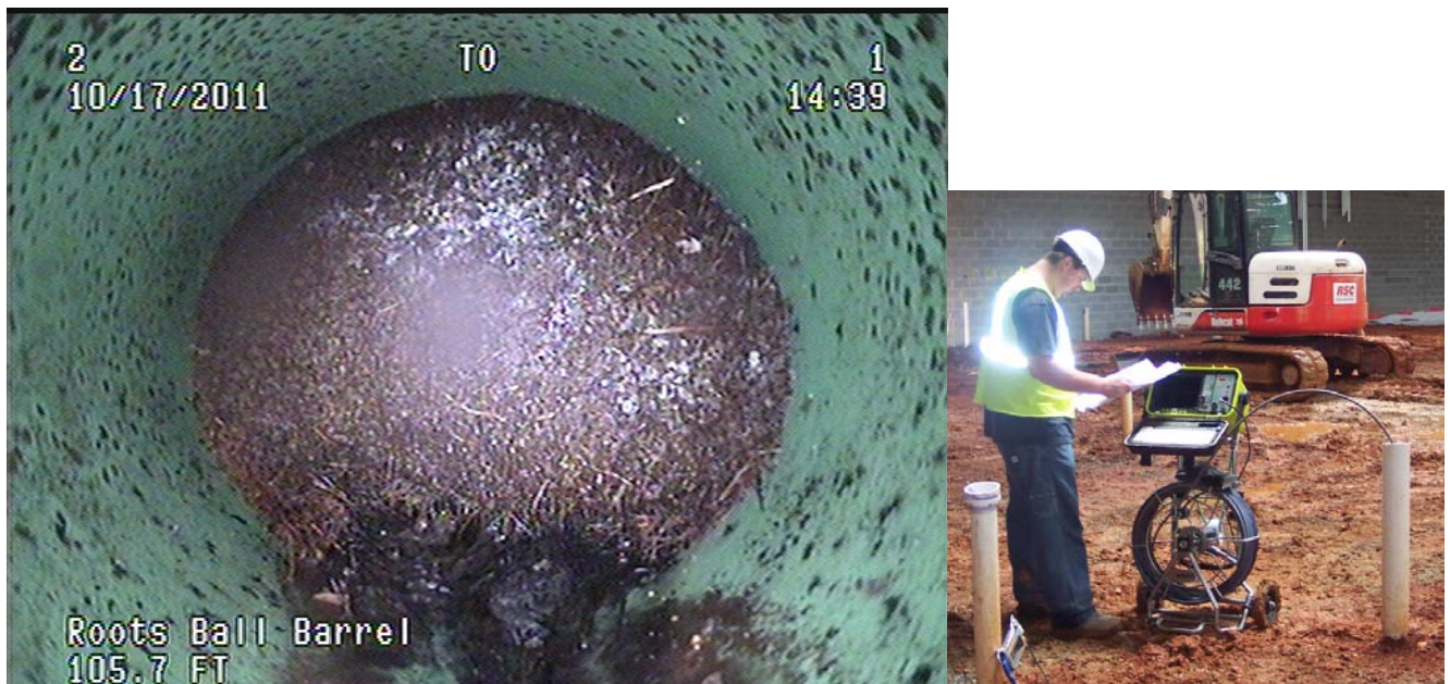
Figure: 7-33. Root mass in a sewer line (left). Camera equipment that photographed this root mass (right). (Trent Warner, PE)
