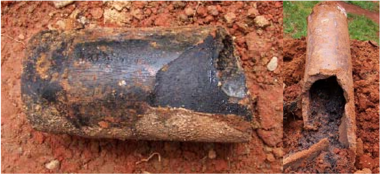
Figure: 7-9. Orangeburg pipe (also known as “fiber” pipe was constructed of paper and tar rolled into a pipe) on the left and terracotta pipe on the right should be replaced with sch 40 plastic pipe. (Photo by Tom Saxton)
