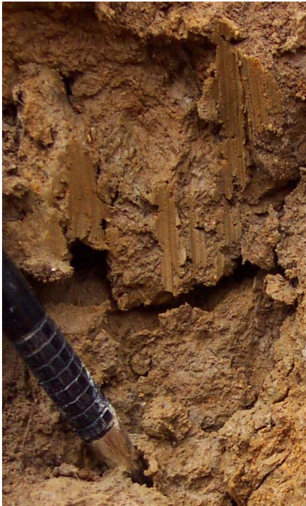
Figure: 4-39. Pressure faces ( stress surfaces ) with (vertical) striations ( slickensides ) shown above the pencil are indicators of high to very high shrink-swell potential. Soils (shrink-swell) with these features are limiting for onsite water treatment.
