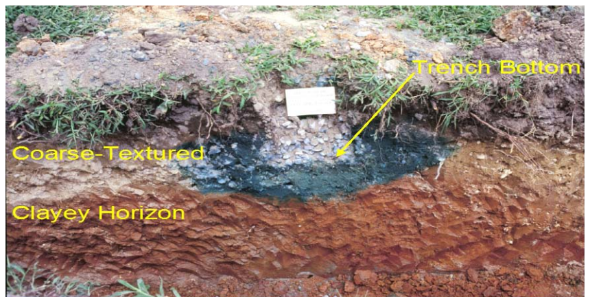
Figure: 5-41. Effluent mounding may occur when the effluent is discharged into a coarse textured soil overlying a fine texture soil horizon. (NCSU)
