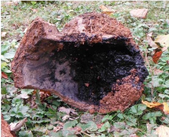
Figure: 7-15. Infrequent septic tank pumping has promoted sludge accumulation in this pipe. (Photo by Sarah Lewis, EHS)
