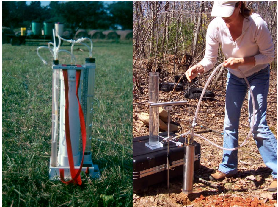
Figure: 5-38. Two types of constant head permeameters commonly used in Virginia; the Amoozemeter (left) and the Johnsonmeter (right). (Photos by Tom Saxton)
