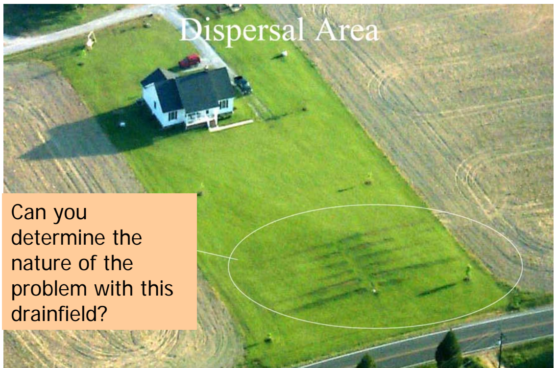
Figure: 7-28. What's wrong with this picture? Lack of equal distribution; the distribution box needs adjustment. Some trenches are receiving more effluent than others. This may shorten the lifespan of this drainfield. The drainfield also appears to be failing over some of the trenches as evidenced by the dead spots where flooding effluent has killed the grass. The distribution box is leaking as well. (Photo by Loudon County EH)
