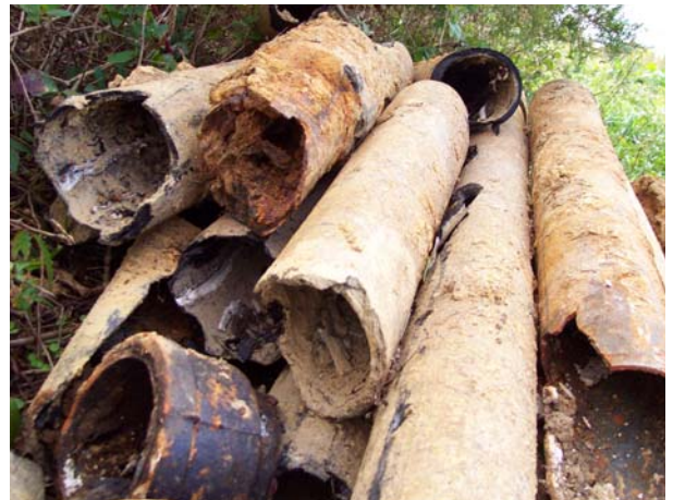
Figure: 7-11. Old cast iron and orangeburg have degraded. (Photo by Tom Saxton)
