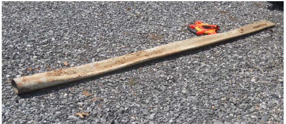
Figure: 7-10. Somehow, this crushed conveyance line lasted 20 years. While the regulations allow this grade of pipe, sch 40 is recommended. (Photo by Tom Saxton)
