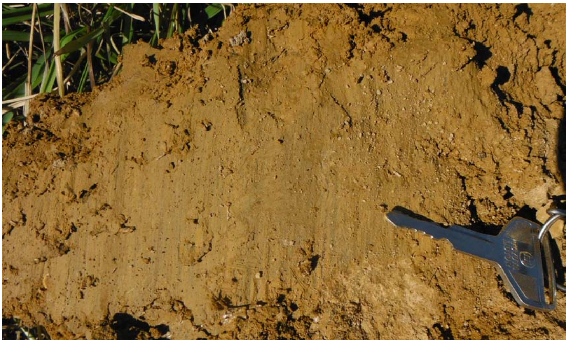
Figure: 6-16. The presence of slickensides indicates smectitic clays that have a high or very high potential for shrinking and swelling. (Photo by Tom Saxton)
