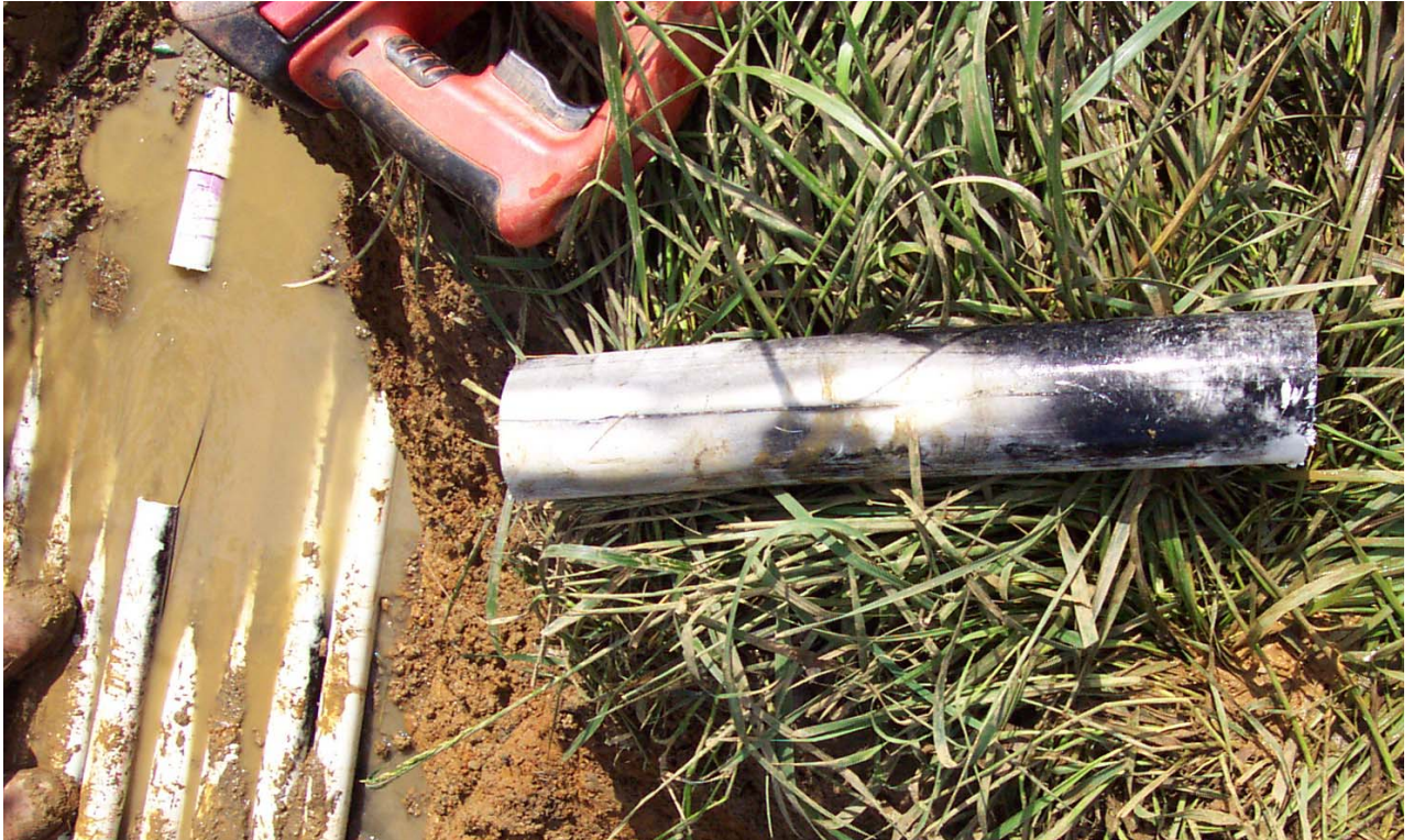
Figure: 7-24. This force main, one of 11, was found to have a linear crack. The difficulty in this case was that all 11 were installed in an easement leading to offsite drainfields. Therefore, 11 homes owned the easement. Who was responsible? Sewage was flowing on the ground. But there was no one to hold responsible in order to repair the failed force main. Ultimately, the original contractors volunteered at their own expense. Offsite systems present unique problems for the evaluator. (Photos by Tom Saxton)
