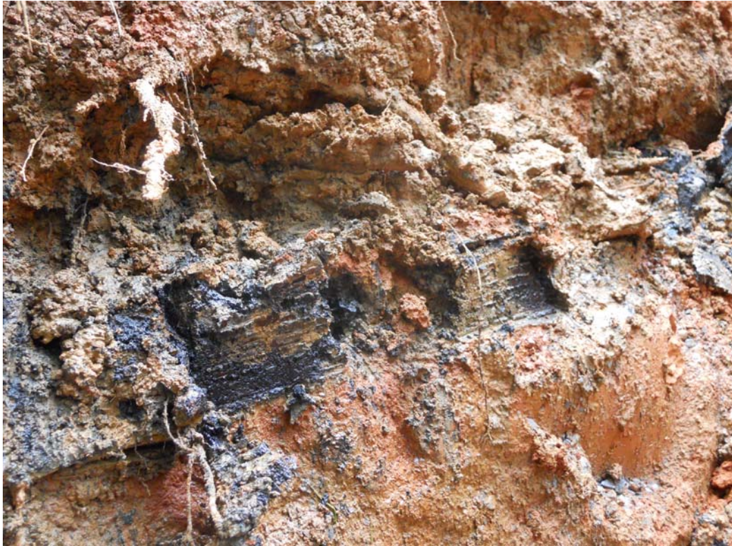
Figure: 7-21. This chamber system is crushed and subsequently filled with soil material. (Photo by Sarah Lewis, EHS)
