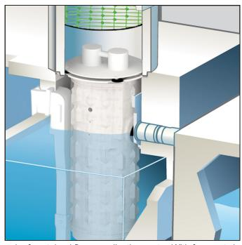
intermittent flow continues to increase, the liquid level may reach a pair of sustained flow equalization ports. With four ports in use, flow through the system increases while continuing to provide flow equalization to all upstream and downstream processes. Peak flow equalization ports are supplied but should not be required in a properly sized system.
