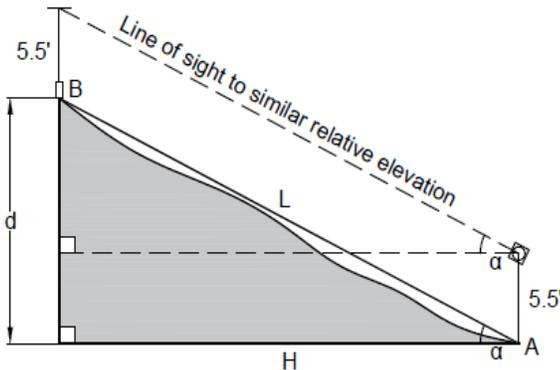
**Step D** – If the clinometer and the point sighted are at the same distance above ground, as shown on the left, this step (Step D Correction) is not necessary.
