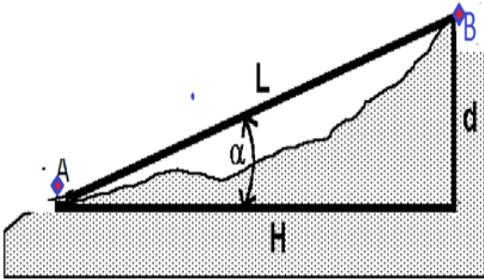
Similarly, you may use a clinometer and a measuring tape to determine the elevation difference between two points. This is essential information when specifying a pump to deliver water or wastewater to a higher elevation. Static or elevation head is the difference between the water level in the pump station and the discharge point of the force main (pump line). The following is a step procedure to determine the elevation difference between two points.
