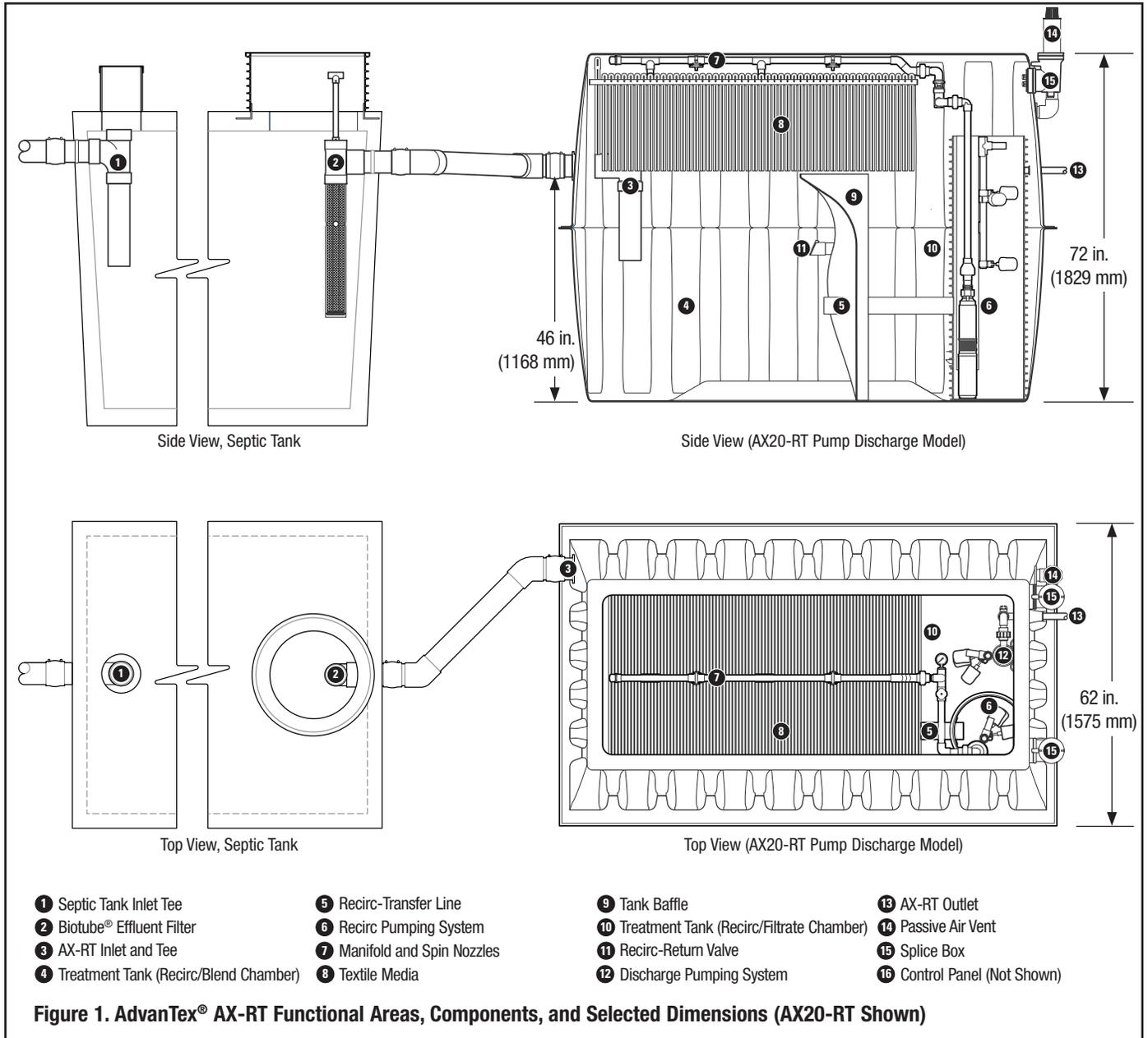
**Figure 1. AdvanTex<sup>®</sup> AX-RT Functional Areas, Components, and Selected Dimensions (AX20-RT Shown)**
