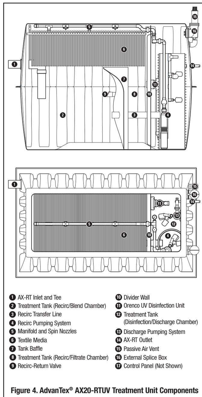
**Figure 4. AdvanTex® AX20-RTUV Treatment Unit Components**
