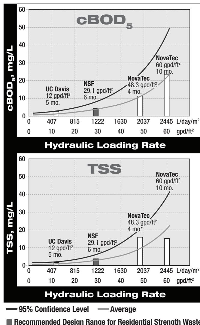
Figure 3. Effluent Quality vs. Hydraulic Loading Rates, Third Party, NSF/ANSI Standard 40 Testing
