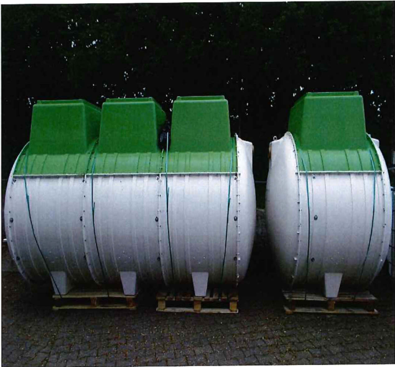
Figure 2: The Tricel Seta plant as delivered on the PIA testing field / before installation
