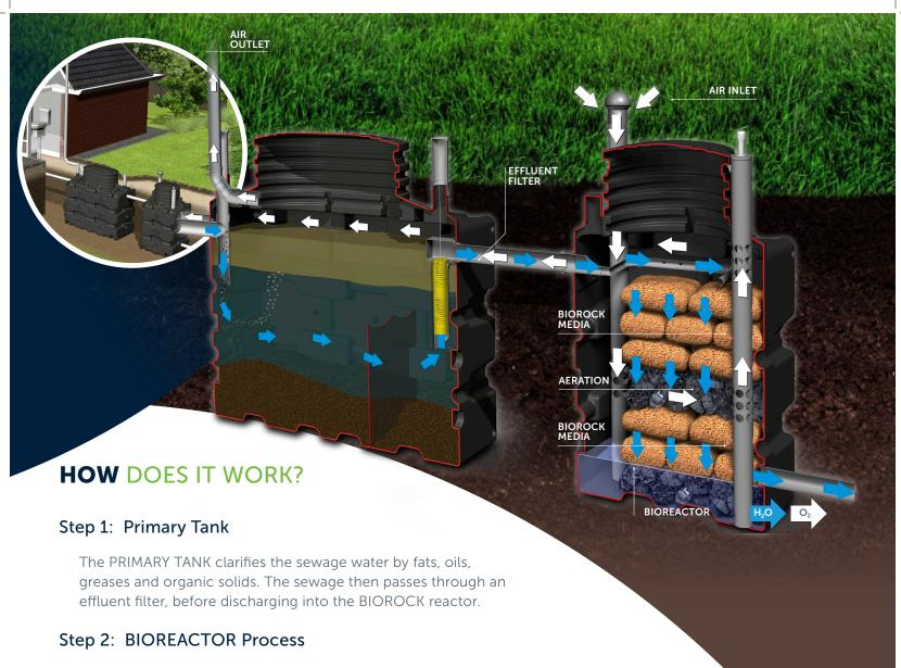
Our BIOREACTOR further purifies the pretreated wastewater using a biological process.
