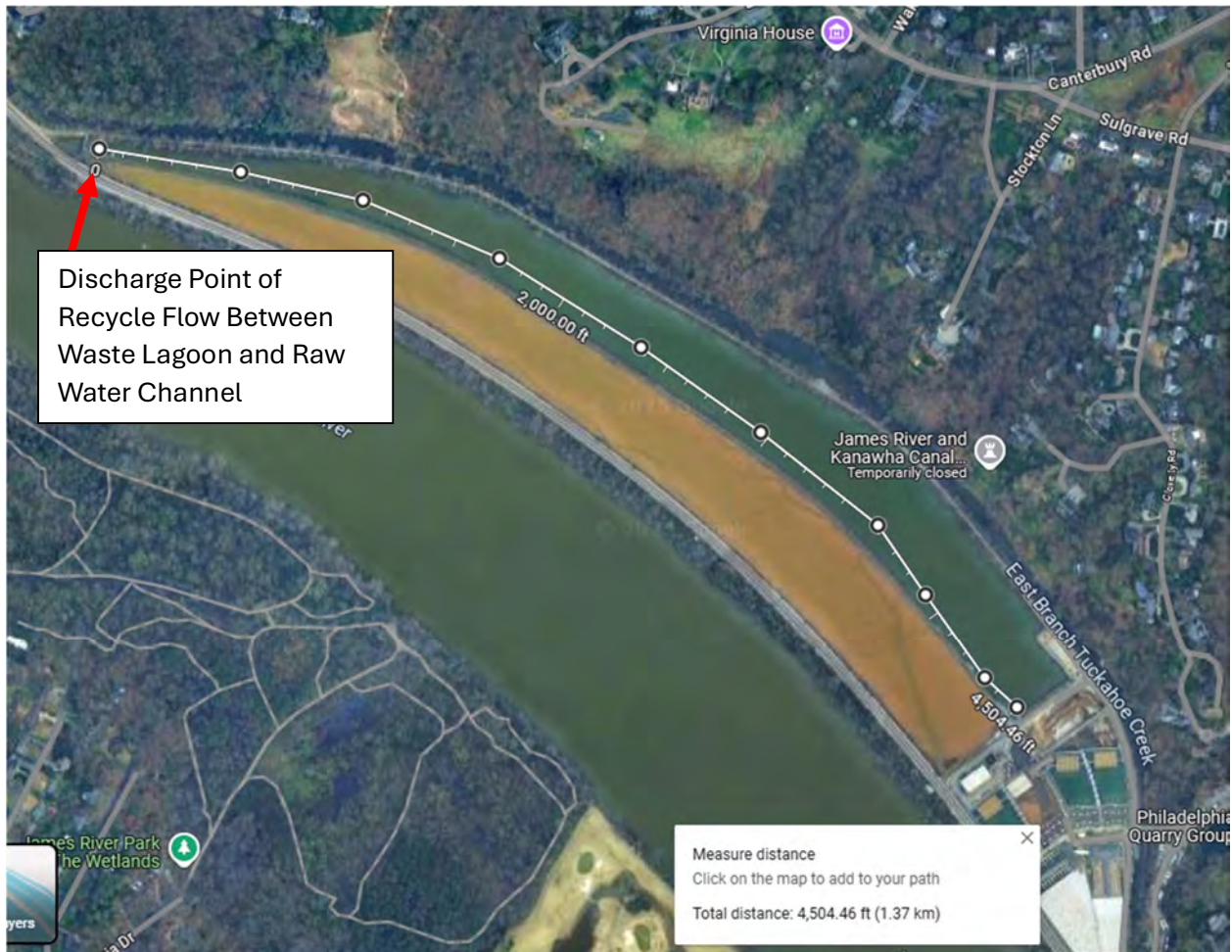
Figure 1. Distance of recycle discharge point and head of raw water pump stations (VDH)
