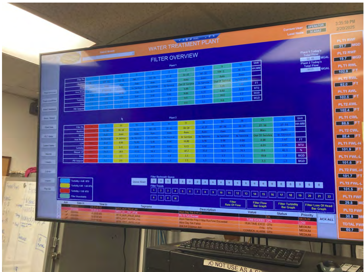
Figure 56. Filters in service/out of service (VDH)
